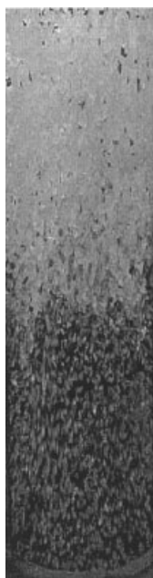
Figure 3. Image of a completely segregated bed for a binary PVC/PC mixture.
